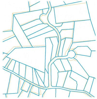
Digital and paper surveys, as well as deeds, provided metes and bounds that were entered to draw improved property lines wherever those sources existed. The less accurate lines from hand-drawn maps (orange) were replaced by the surveyed lines (blue).
