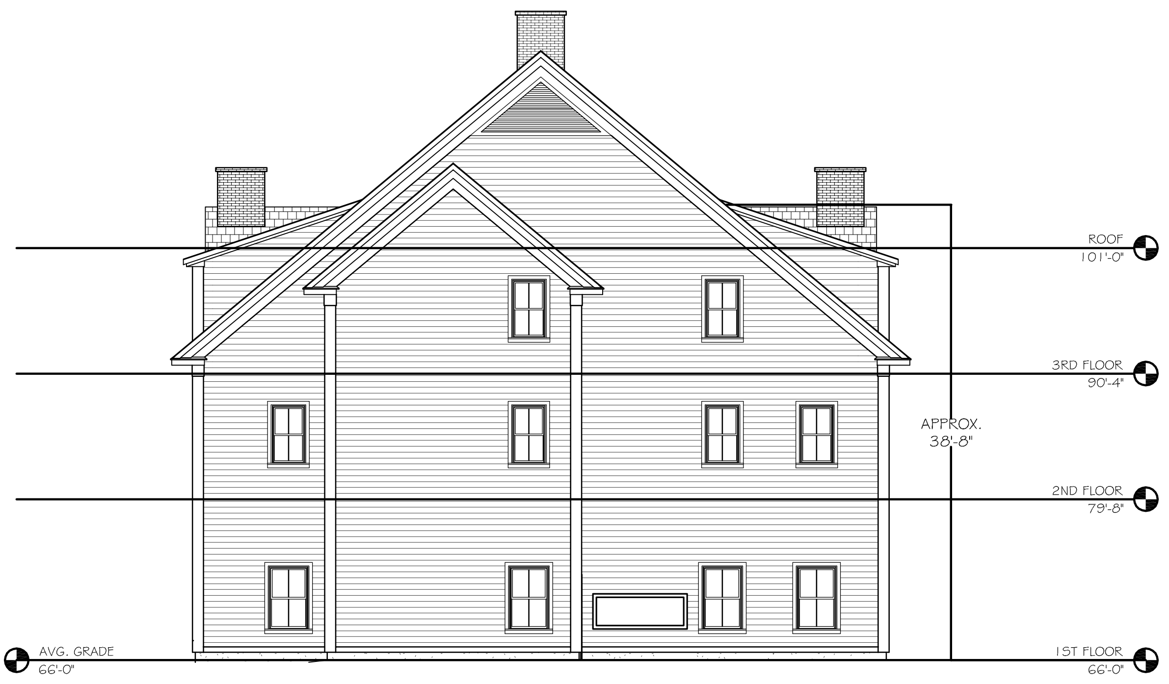
Building A South Elevation 1/8" = 1'-0" 2
