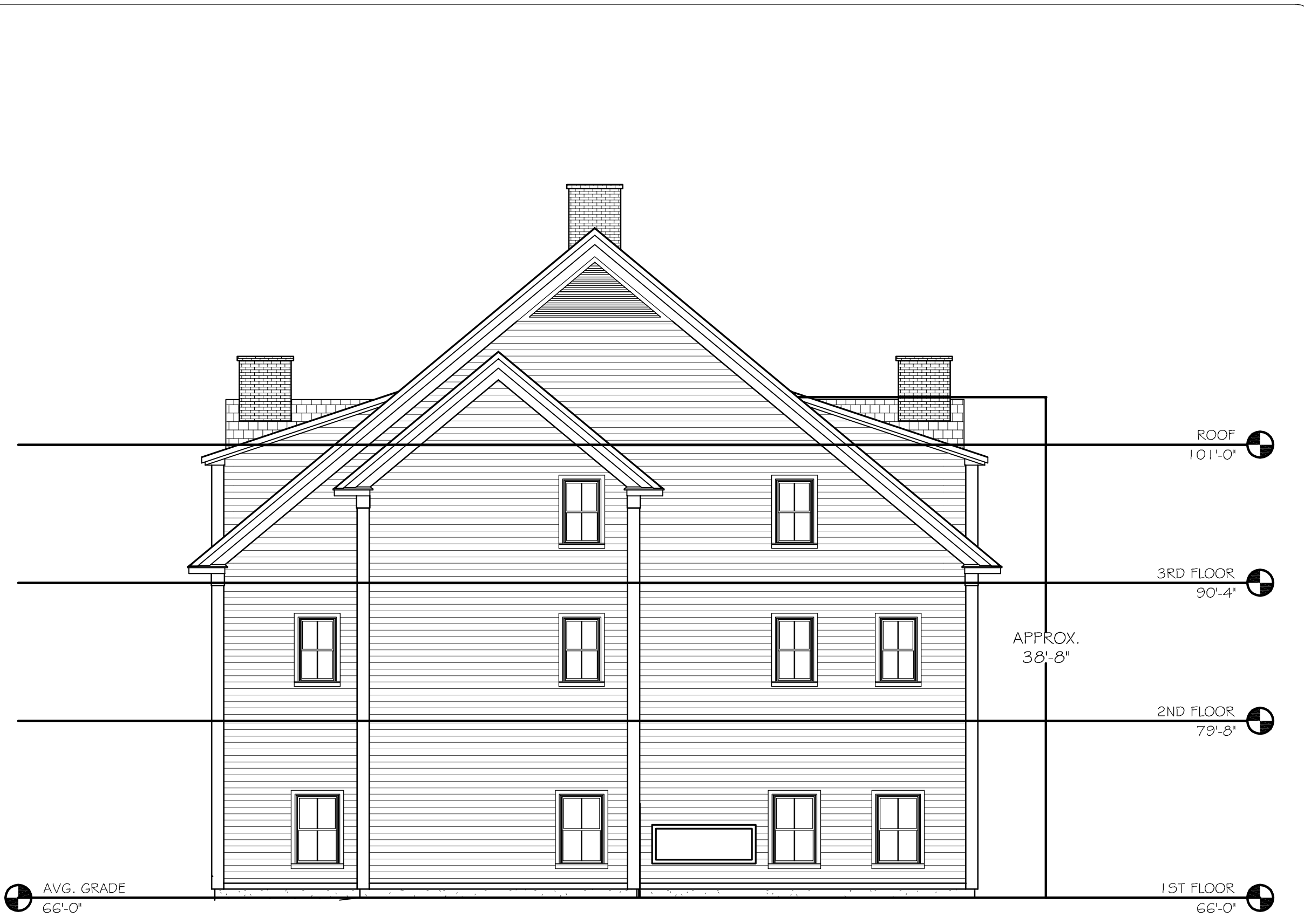
Building A South Elevation 1/8" = 1'-0" 2
