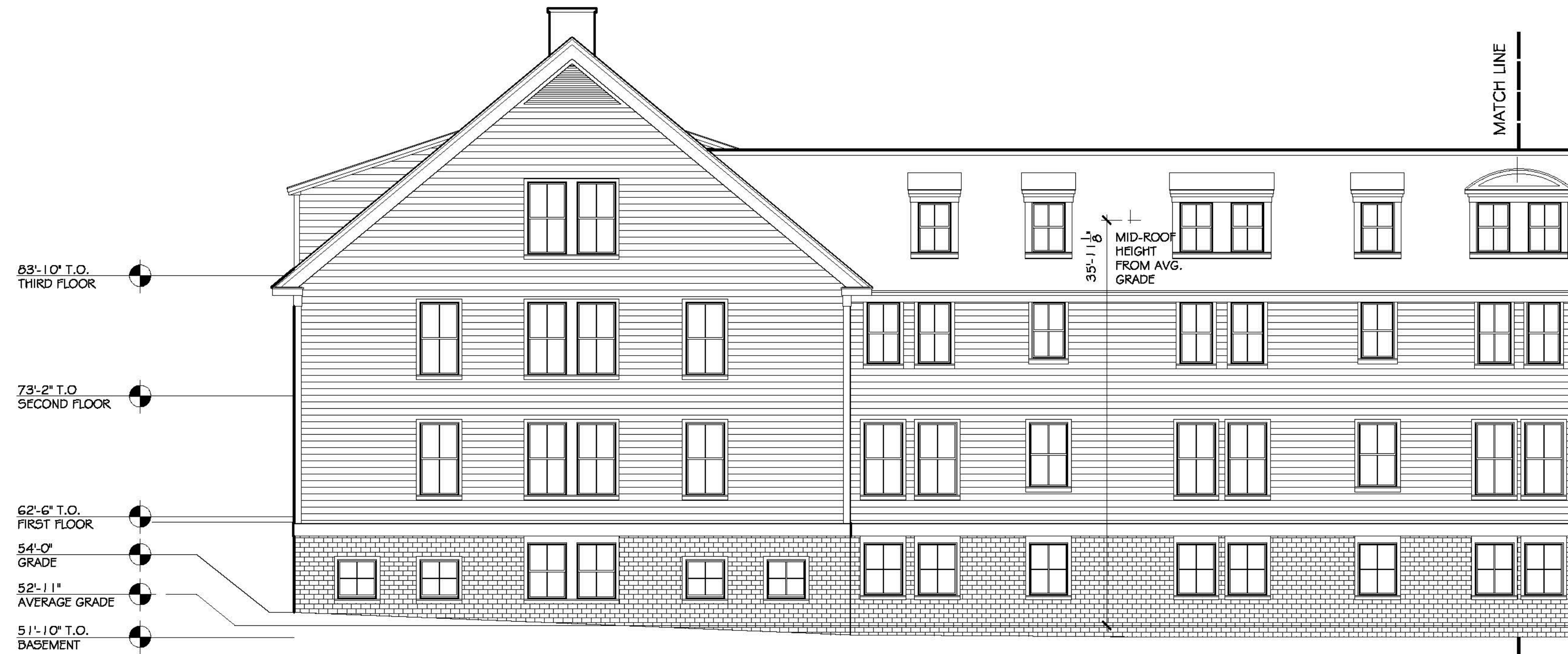
Building B South Elevation 2 1/8" = 1'-0" 2
