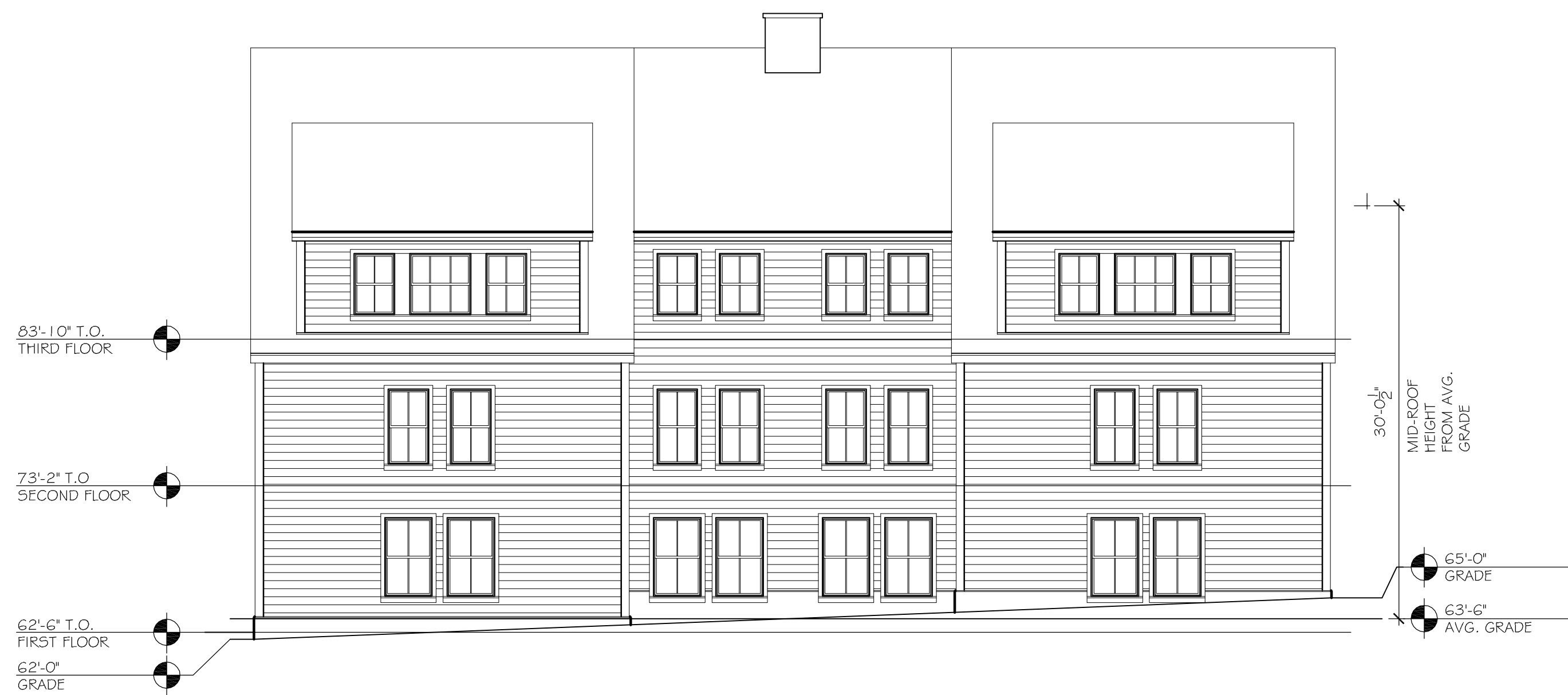
Building B East Elevation 1/8" = 1'-0" 4
