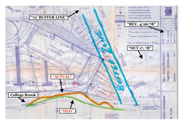
In addition, some discrepancies between site plan and field measurements were significant. It would appear that the edge of pavement toward Church Hill encroached into the 75-foot buffer to the residential zone. (See the comparison of site plan and field measurements on the detail from the "Parking Improvement Plan" dated June 25, 1979, below.)
